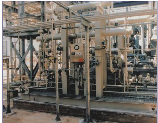
Figure 6. A hydrocarbon recovery unit.
