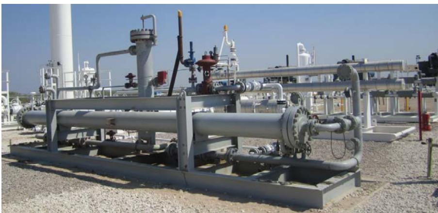
**Figure 2.** Block diagram and photograph of a membrane FGCU used for a gas gathering compressor engine in the Eagle Ford Shale, TX. The membrane modules are contained in the horizontal pressure
