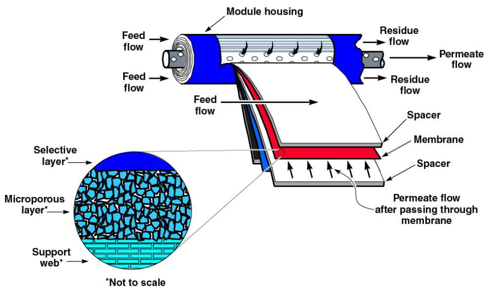
**Figure 1.** Schematic illustrations of a composite membrane and a spiral-wound module of the type used in fuel gas conditioning units.
