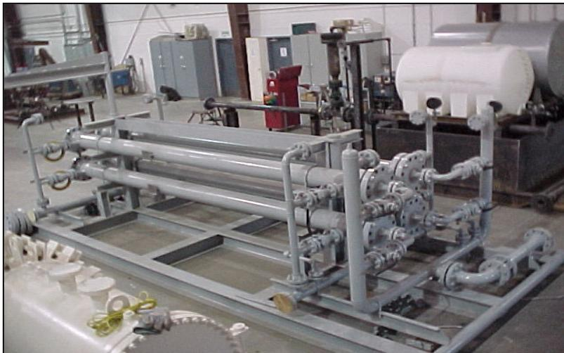
**Figure 5.** Photograph of FGCU designed to treat high hydrogen sulfide-content gas. Skid mounted with four horizontal pressure vessels shown in the photograph.
