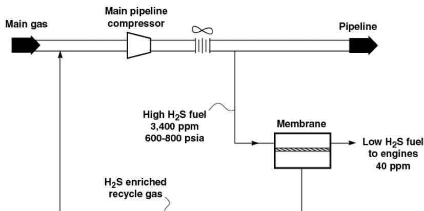
**Figure 4.** Block flow diagram and photograph of FGCU designed to treat high H<sub>2</sub>S-content gas.
