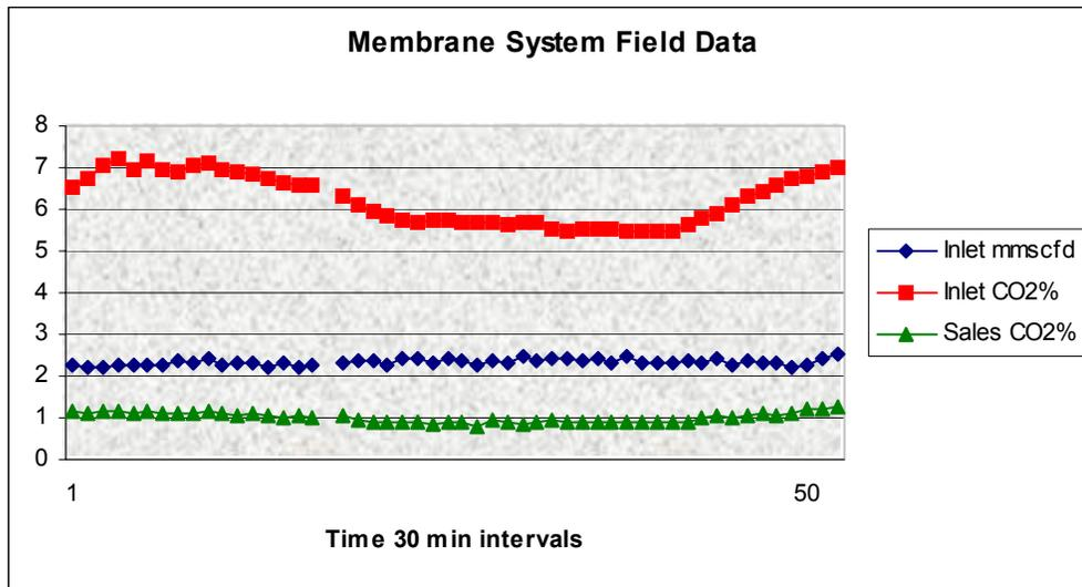
**Figure 6. Field performance data for operation of a membrane CO<sub>2</sub> removal system (Dominion's Alverstone unit near Sheridan, Texas).**
