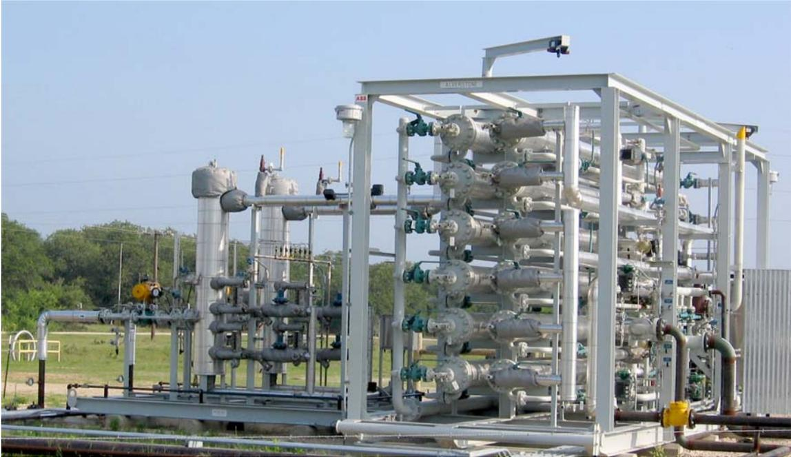
**Figure 4. A standard CO<sub>2</sub> treatment skid with pretreatment filter/separators on adjacent skid to left.**
