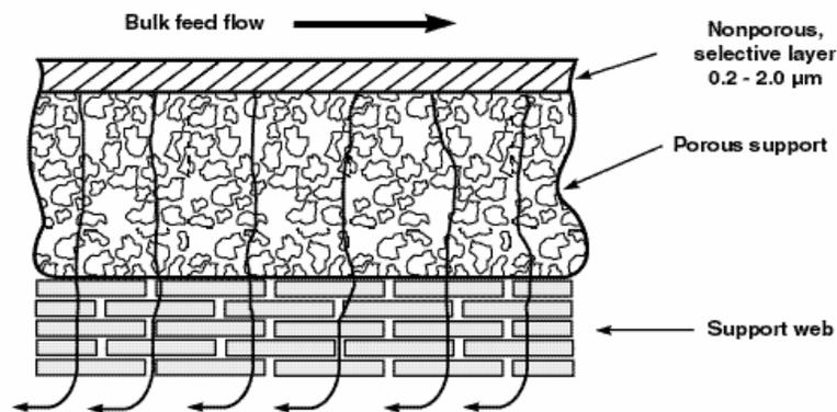
**Figure 1. Cross-section of an MTR composite membrane.**
