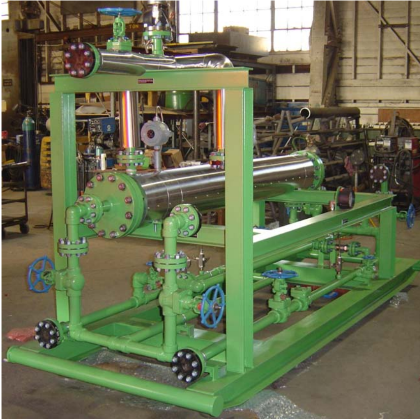
Twin Bottoms Membrane System Design Flow Rate-0.2 MMSCFD
