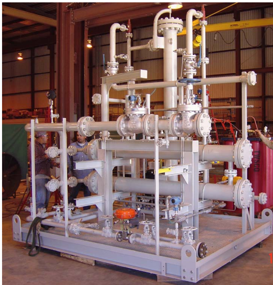
Figure 12. Flow diagram and shop photograph of a membrane fuel gas conditioning unit used for a field gas compressor engine. The membrane modules are contained in two horizontal pressure vessels. The unit can produce 0.5 to 1.0 MMscfd of clean gas.
