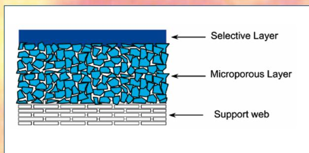
Figure 1. The VaporSep membrane.
