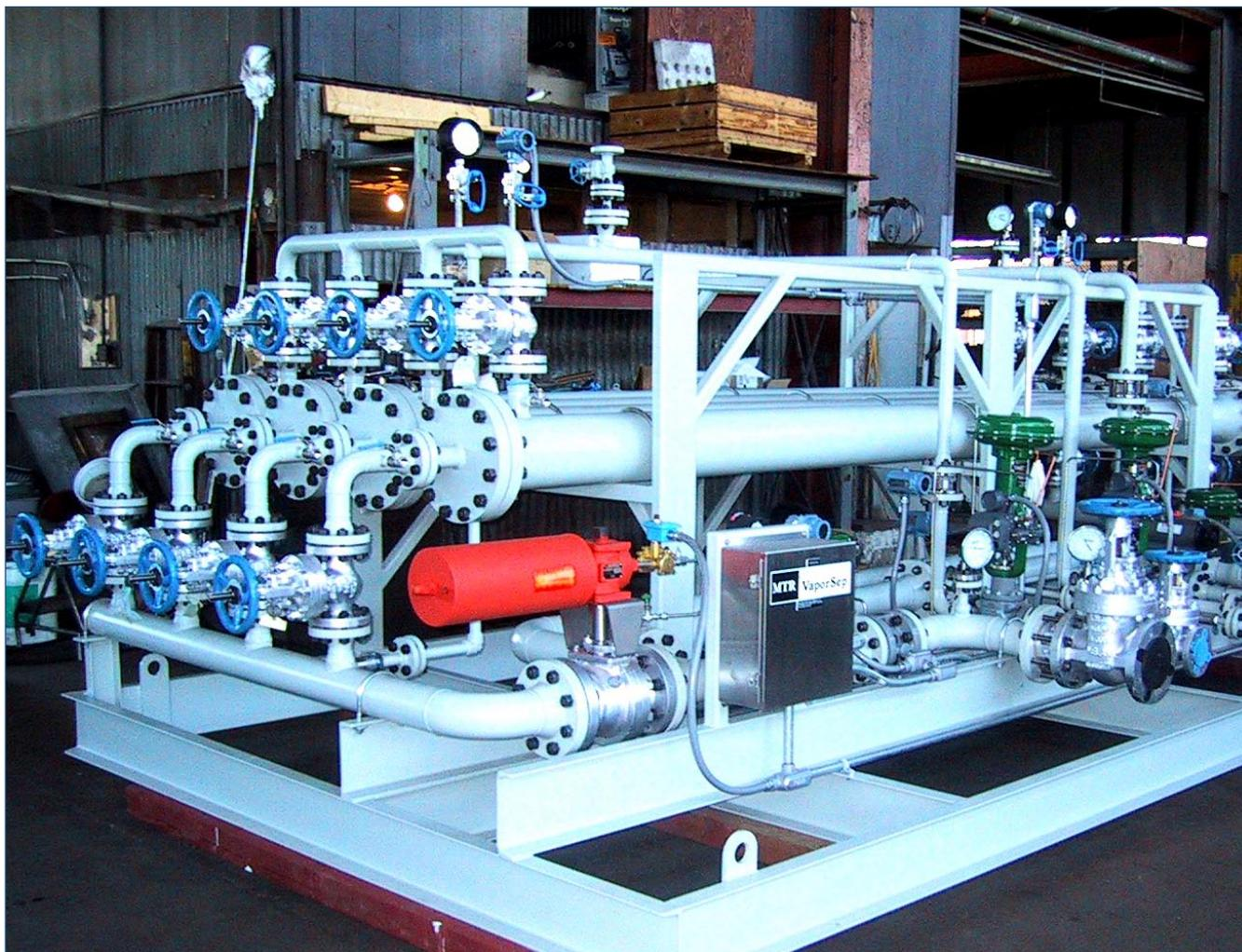
**Figure 4. An ethylene recovery unit.**
