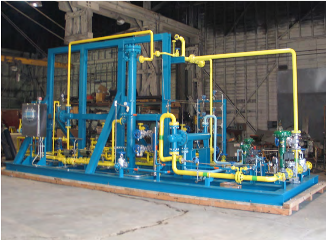
VaporSep-H 2 ™ system for hydrogen recovery from methanol plant purge gas
