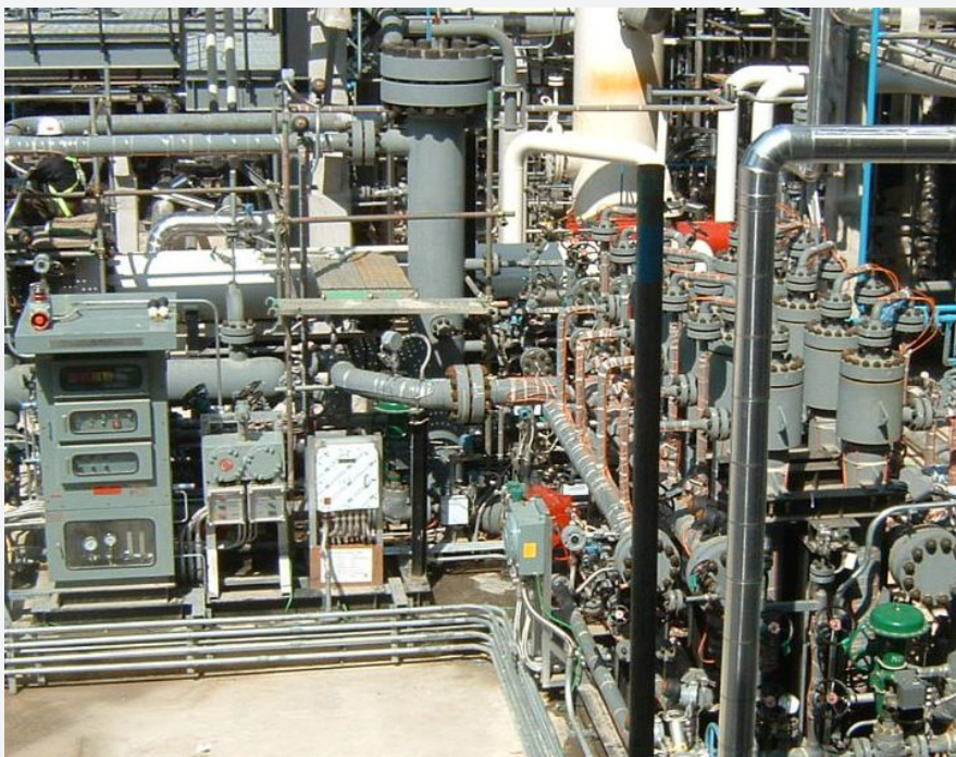
This VaporSep-H 2 ™ unit recovers hydrogen from hydrotreater offgas in an Asian refinery
