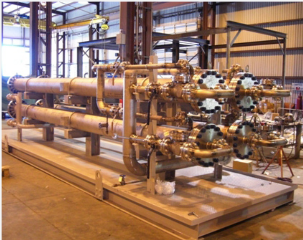
SourSep™ unit for installation on an Indonesian remote production field
